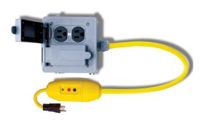
The inline GFCI version of our 14880 quad boxes, these units offer convenient safe power distribution for heavy power users. GFCI has lighted power-on indicator. Good for indoor and outdoor use. Units come in both 15A and 20A versions and have 12/3 SJTW cord.
