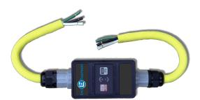
Pre-set trip levels and two feet line and load cord, these units support single phase power across a range of voltages. Dual LED indication lights display power and fault status. All units are automatic reset and NEMA 4X rated. Manual reset versions available upon request.
