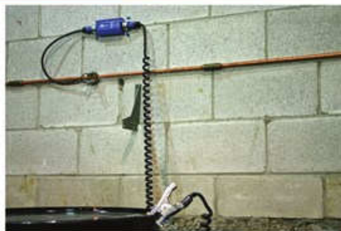
Linde Equipment's StaticSure portable static monitoring system is shown here monitoring a barrel.
