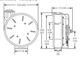
Our LE9000 series of reels are built with durable all-steel weatherproof (NEMA 4 enclosure) construction so that they will survive in the toughest work environments. We've built the cable guide arm with thicker steel than our competitors to take extra abuse. All this while still keeping the form factor small so that your reel isn't always in the way.
